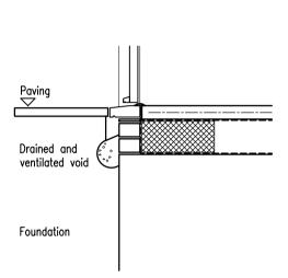
Flush Threshold Detail 0 0.2 0.4 0.6 0.8 1.0
